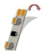
2. Peel off the 3M isolation tape from the light strip.
