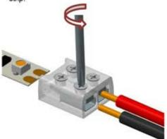
Loosen the screws to peel off the outer rubber of the light strip and wire and insert it into the connector (note: the positive and negative poles of the light strip in both directions should correspond).
