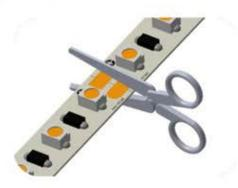
Unfold the light strip and cut the required length, cut it from the cutting place of the light strip.
