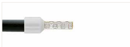
Tin-plated copper ferrule (gas-tight crimped)
