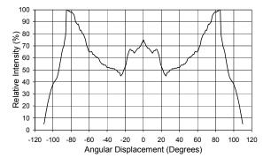
Figure 6. Representative Typical Spatial Radiation Pattern for Luxeon V Star.
