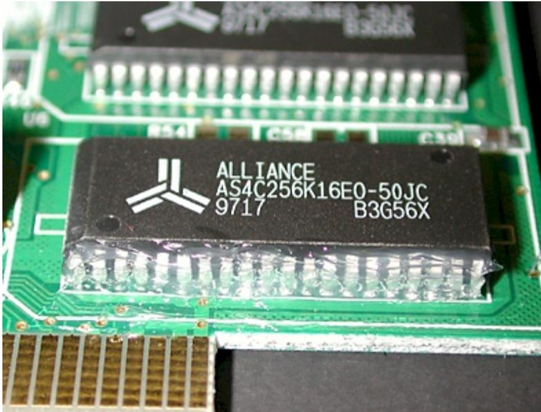
d. If you have doubts about your ability to apply the silicone to the chip leads without getting it all over the top of the chip, cover the top of the chip with a piece of masking tape before you apply the silicone.
