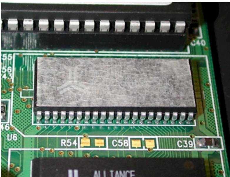
e. Apply the silicone as in "b" above. Wipe the silicone that gets on the masking tape off with a rag or paper towel before it sets. Once the silicone has had at least one hour to set, carefully remove the masking tape and check the mating surface of the chip as detailed in "c".
