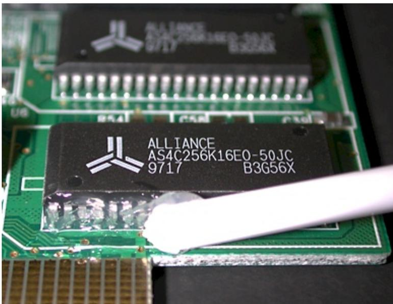
c. Wait the appropriate amount of time for the silicone to set completely per its instructions. When it is set, make sure that the mating surface of the chip is clean and that there is not any silicone strands that will interfere with the heatsink mounting.
